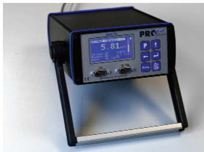
Fig. 2 — Newer zirconium oxide cell oxygen indicators, such as this Pro2-plus from Intercon Enterprises, offer fast warm-up times, robust housings, and the ability to measure oxygen levels as low as 1 ppm.
